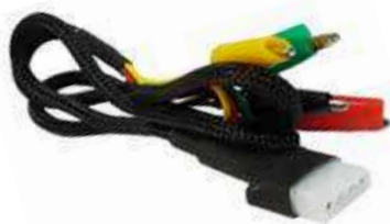
Fig. 4. Four-wire diagnostic cable.
