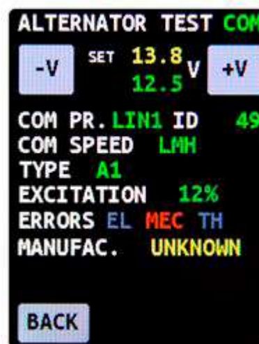
Fig. 7. Diagnostic window of the “COM”-type alternator.
